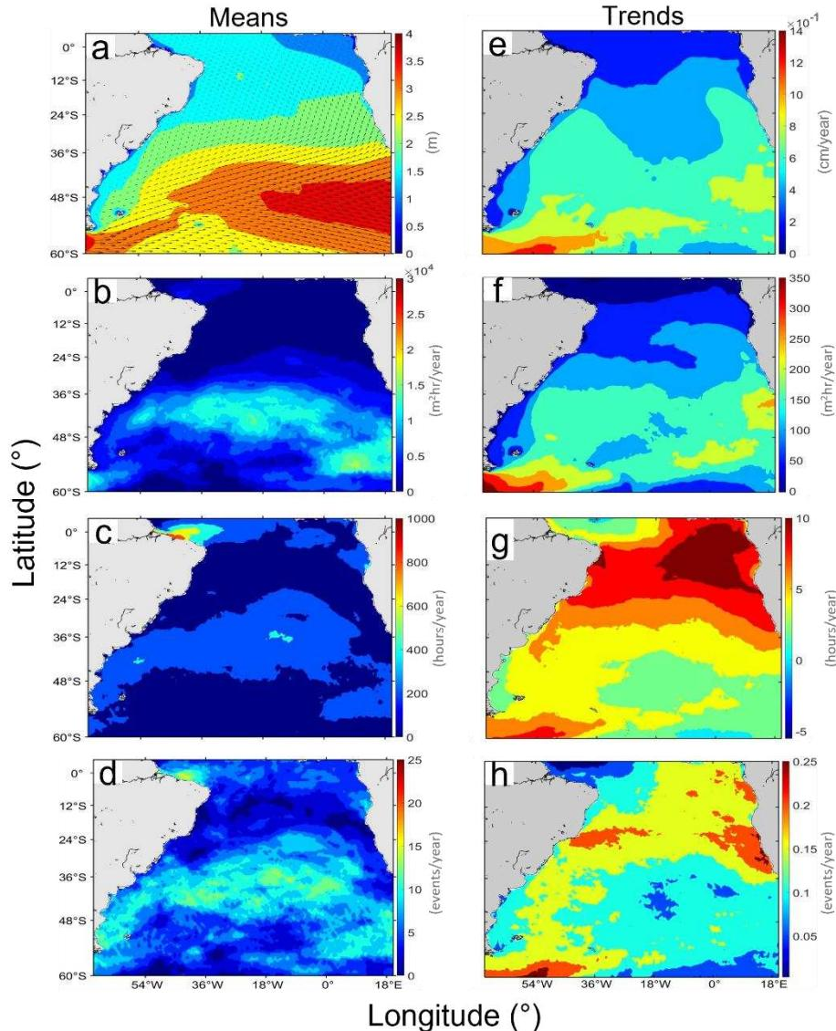
**Figure 2.** Time-average (left-hand panels) and trend (right-hand panels) of  $H_s$  and extreme event parameters between 1950 and 2021: (a,e)  $H_s$ ; (b,f) cumulative Intensity; (c,g) cumulative Duration; (d,h) Frequency.
