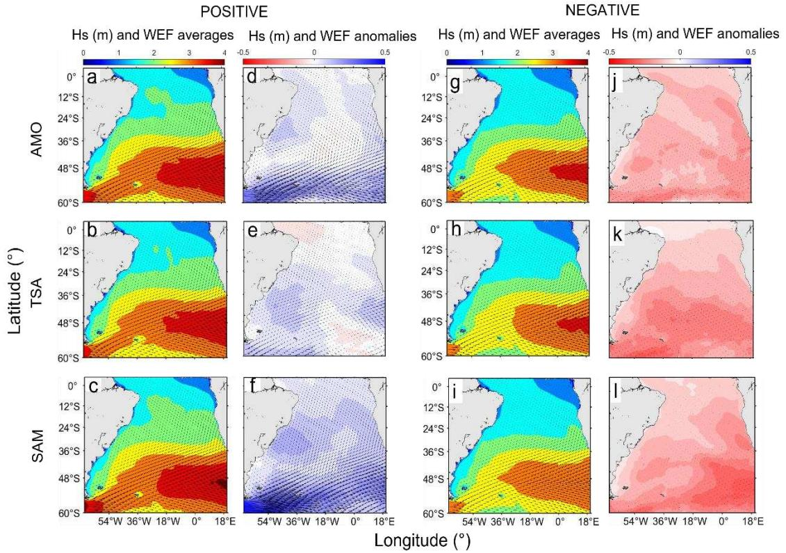
**Figure 5.** Mean  $H_s$  and  $WEF$  and corresponding anomalies over the 5 most (left-hand panels, positive phase) and less (right-hand panels, negative phase) intense years of each climate index.
