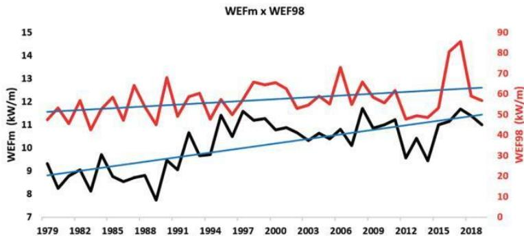
**Figure 3.** WEF variation between 1979–2019. The black and red lines indicate WEFm and WEF98 variations during all analyzed periods, respectively. The blue continuous lines indicates the significant growth trend of the WEFm and WEF98. WEFm=mean wave energy flux; WEF98= extreme wave energy flux (98<sup>th</sup> percentile).
