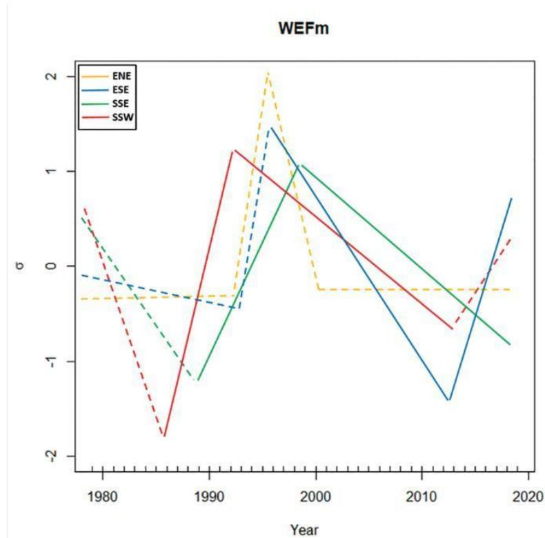
**Figure 6.** WEFm variation per quadrant. Continuous lines indicate subperiods with significant variations, and segmented lines indicate subperiods without significant variations. WEFm=mean wave energy flux.
