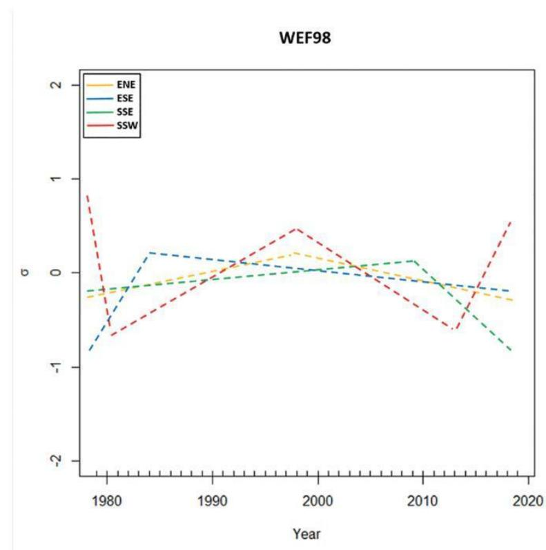
**Figure 7.** WEF98 variation per quadrant. Segmented lines indicate subperiods without significant variations. WEF98= extreme wave energy flux (98<sup>th</sup> percentile).
