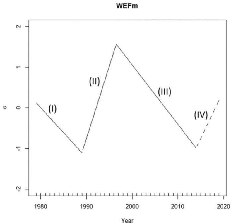
**Figure 4.** Segmented linear model of the normalized residuals from WEFm linear models. Continuous lines indicate subperiods with significant variations and segmented lines indicate subperiod without significant variations. WEFm=mean wave energy flux.
