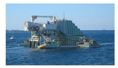
**Figure 2.16:** Oceanlix Mk1 OWC device, in Wollongong, Australia (Falcão and Henriques, 2016).
