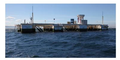
**Figure 2.18:** Mk3 floating platform with multiple OWC chambers at Port Kembla, in Wollongong, Australia (Falcão, 2014).
