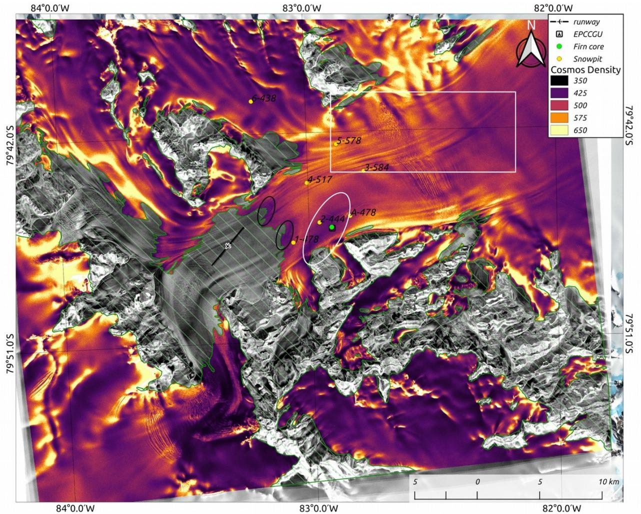
499 Figure 10: Map of the snow density that was derived with a radiative transfer model algorithm applied
