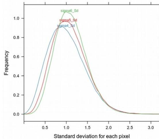
274 Figure 2: Histograms that compare the standard deviations of the averaged images using only the four
