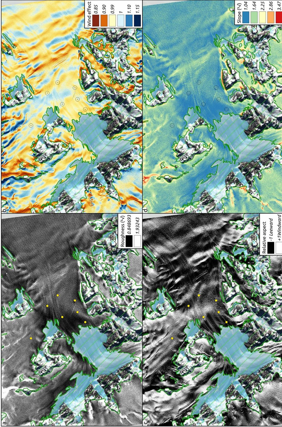
525 62Figure 12: Four derived terrain products: (a.) cube root of the roughness values; (b.) wind effect for a mean wind direction of 255° and search window of 1
